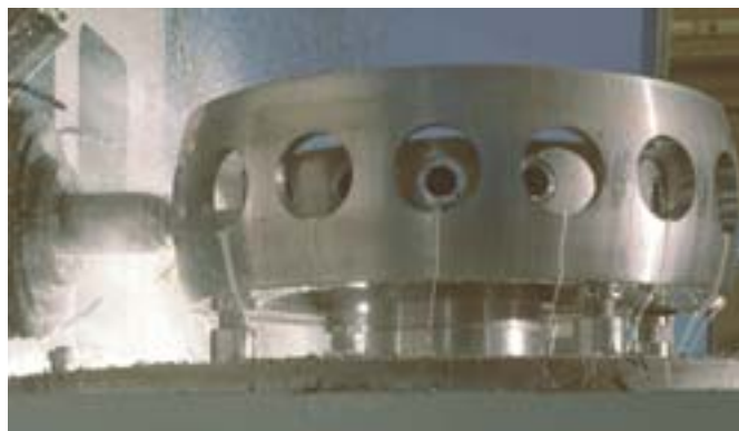
Machining of a Variax™ variable pitch axial flow fan hub in Howden's Belfast facility
