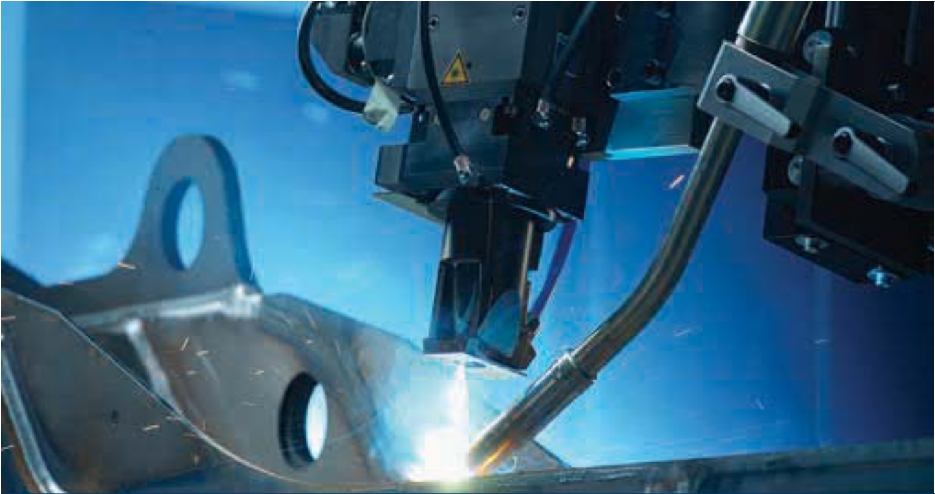
ESAB Laser-hybrid welding machine in action
